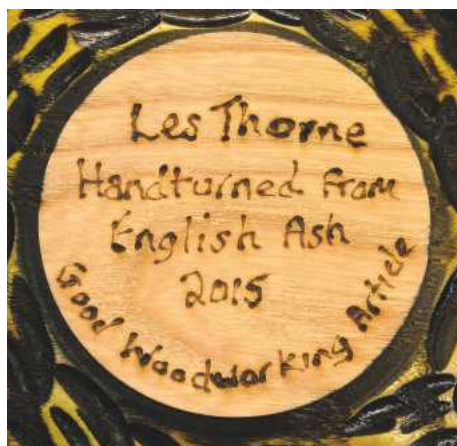
▲ Pic.35 I have signed this using a pyrography machine. Burning a signature into the base is a great permanent record. Lightly sand the surface afterwards to remove any loose burnt bits
